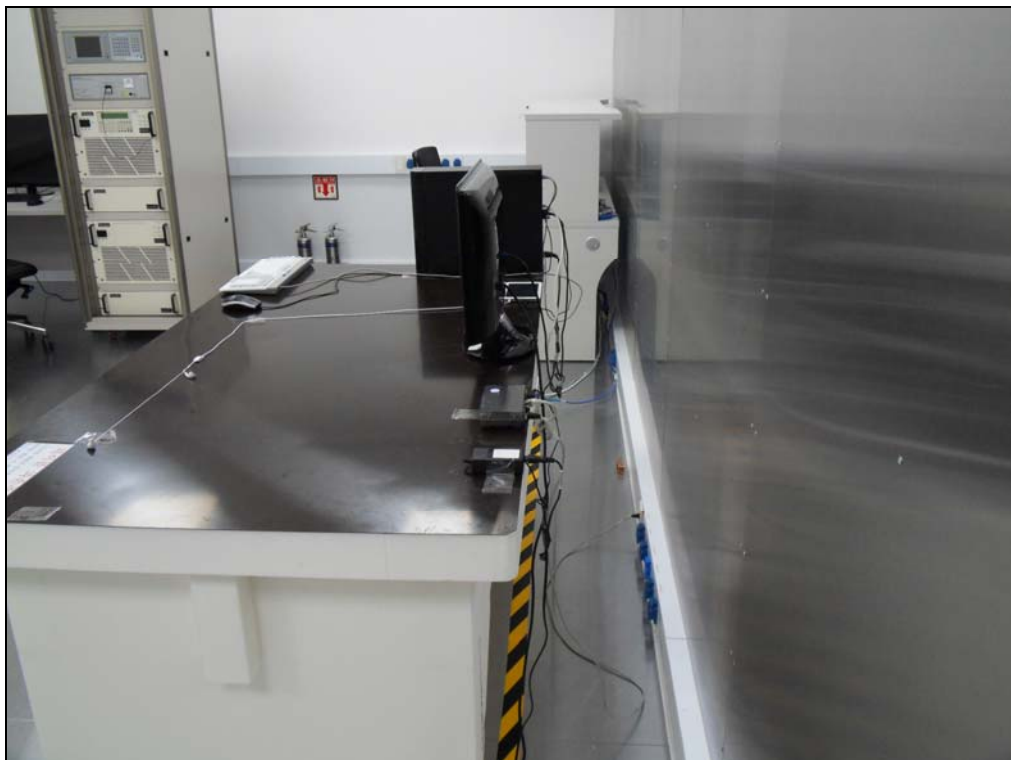
[ Conducted Disturbance – Rear ]
