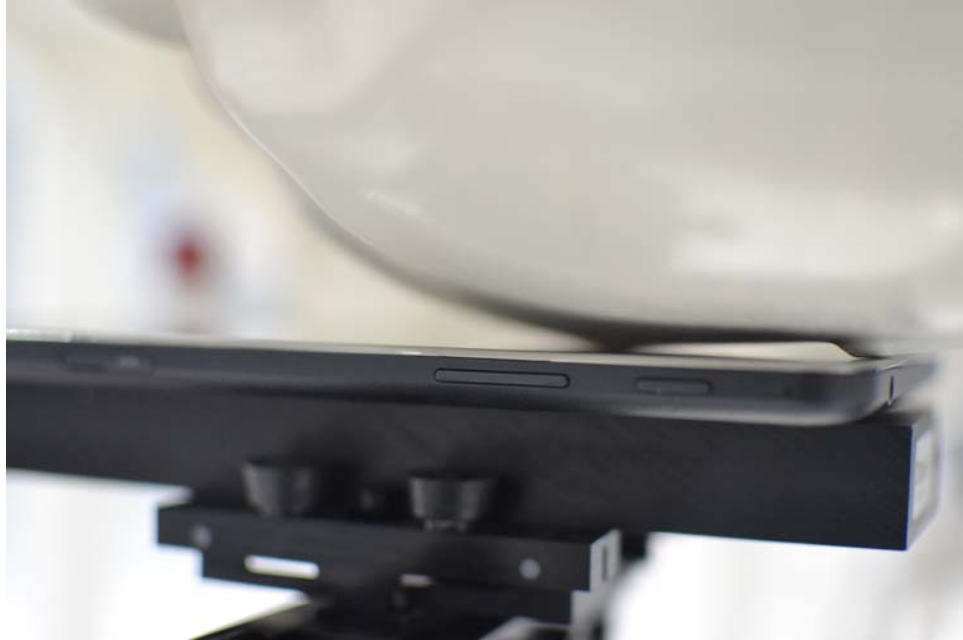
SAR Test Setup Photo 3: Left Cheek
