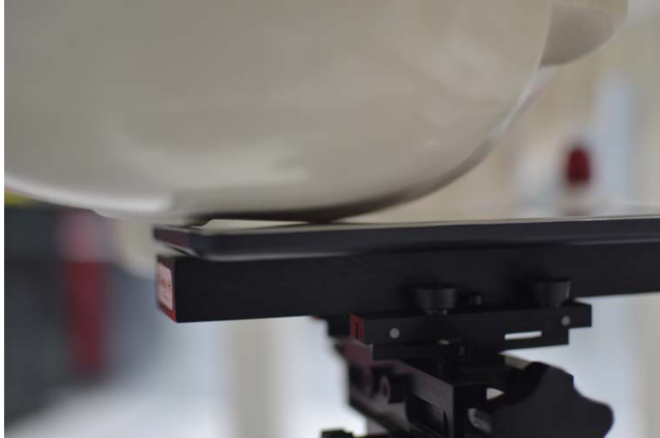
SAR Test Setup Photo 1: Right Cheek
