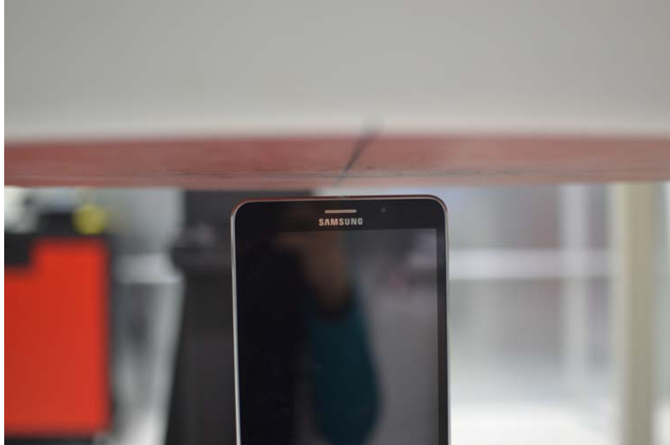
SAR Test Setup Photo 7: Top Edge at 15 mm
