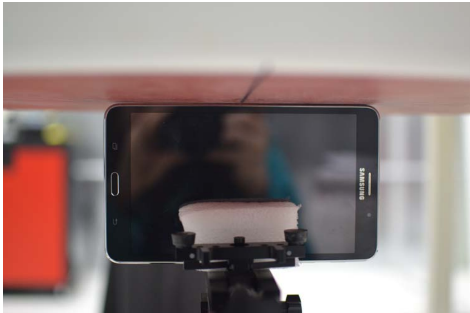
SAR Test Setup Photo 10: Left Edge at 0.0 mm
