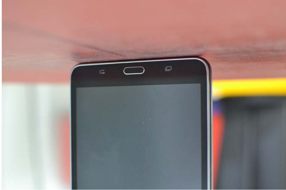
SAR Test Setup Photo 11: Bottom at 0.0 mm
