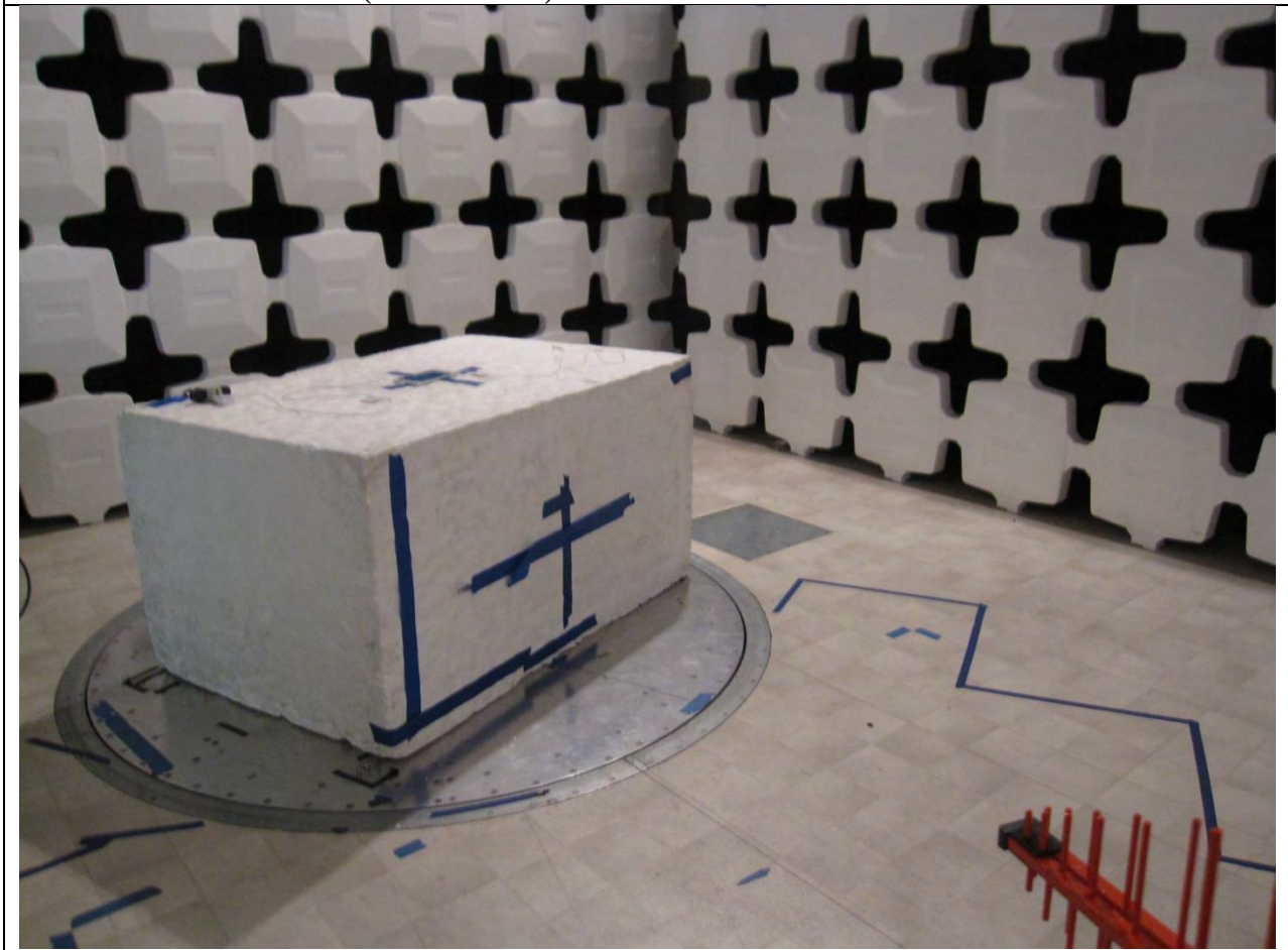
RADIATED FRONT=PHOTO (BELOW 1 GHz)
