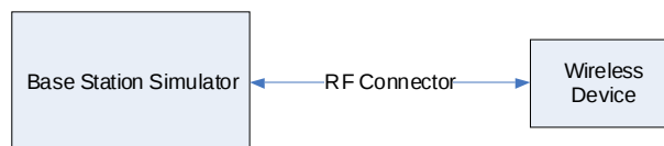
Figure 9-2 Power Measurement Setup
