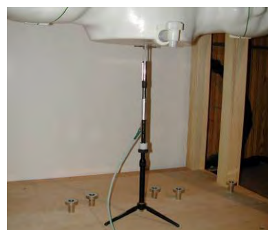
Figure 10-2 System Verification Setup Photo
