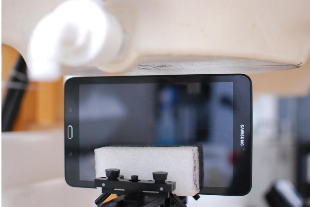
SAR Test Setup Photo 5: Left Edge at 0.8 cm
