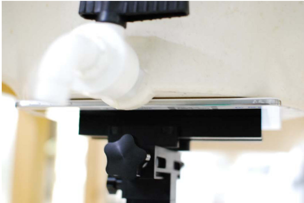
SAR Test Setup Photo 1: Back at 0.0 mm
