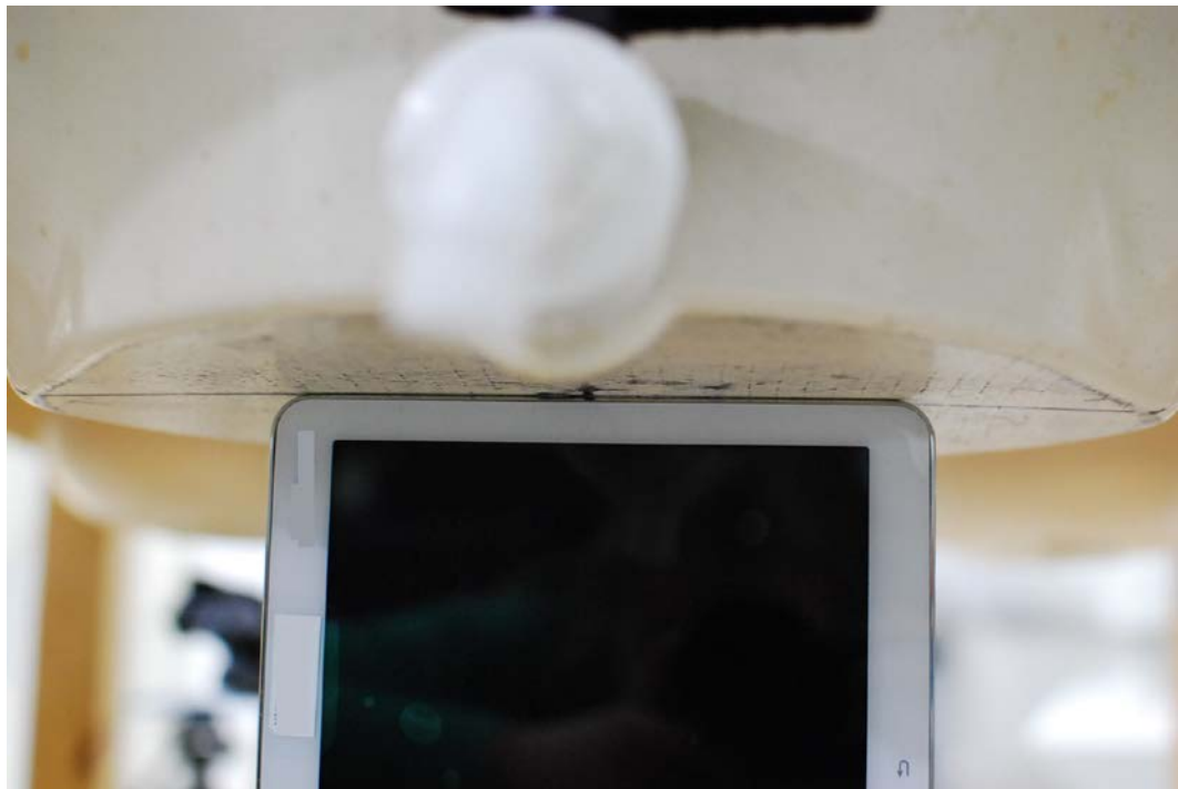
SAR Test Setup Photo 4: Right at 0.0 mm
