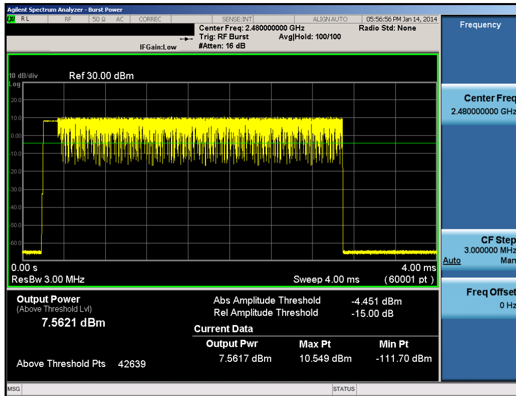
Plot 6-27. Average Conducted Power (3Mbps – Ch. 78)
