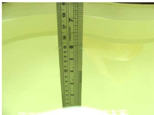
Photo of Liquid Height for Head SAR
