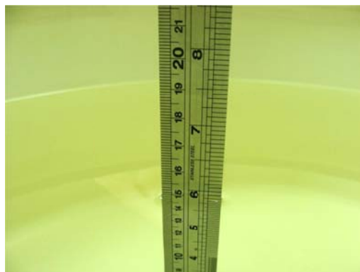
Photo of Liquid Height for Body SAR
