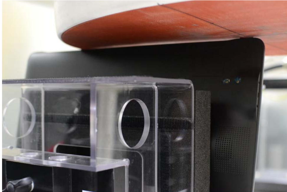
SAR Test Setup Photo 7 – Bottom Edge (Main Antenna) at 0.0 cm
