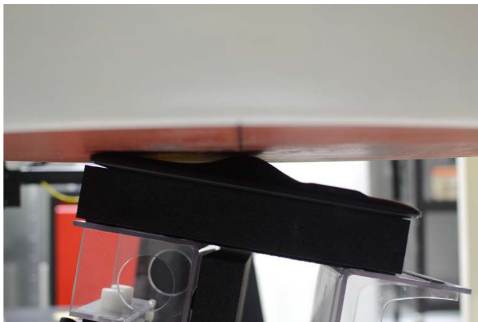
SAR Test Setup Photo 5 – Back Side (Top Touch, WLAN Antenna) at 0.0 cm
