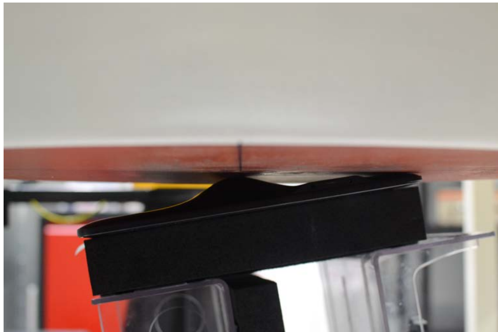
SAR Test Setup Photo 4 - Back Side (Bottom Touch, WLAN Antenna) at 0.0 cm
