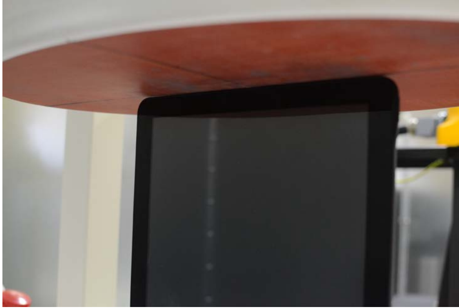
SAR Test Setup Photo 9 – Right Edge (WLAN Antenna) at 0.0 cm
