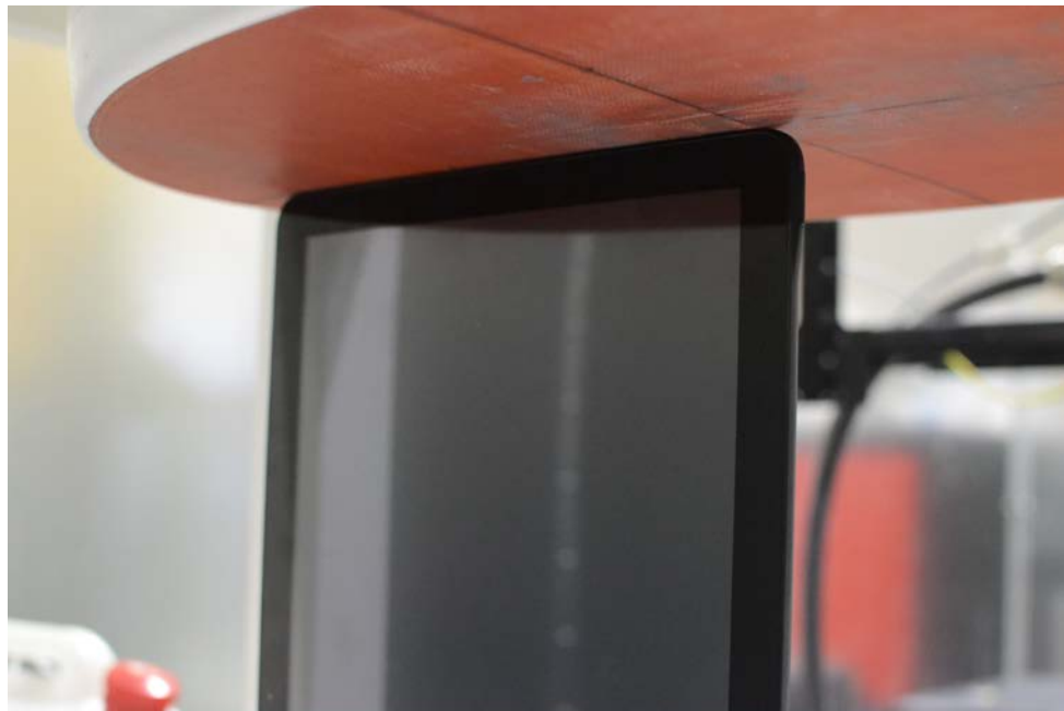
SAR Test Setup Photo 8 – Right Edge (Main Antenna) at 0.0 cm
