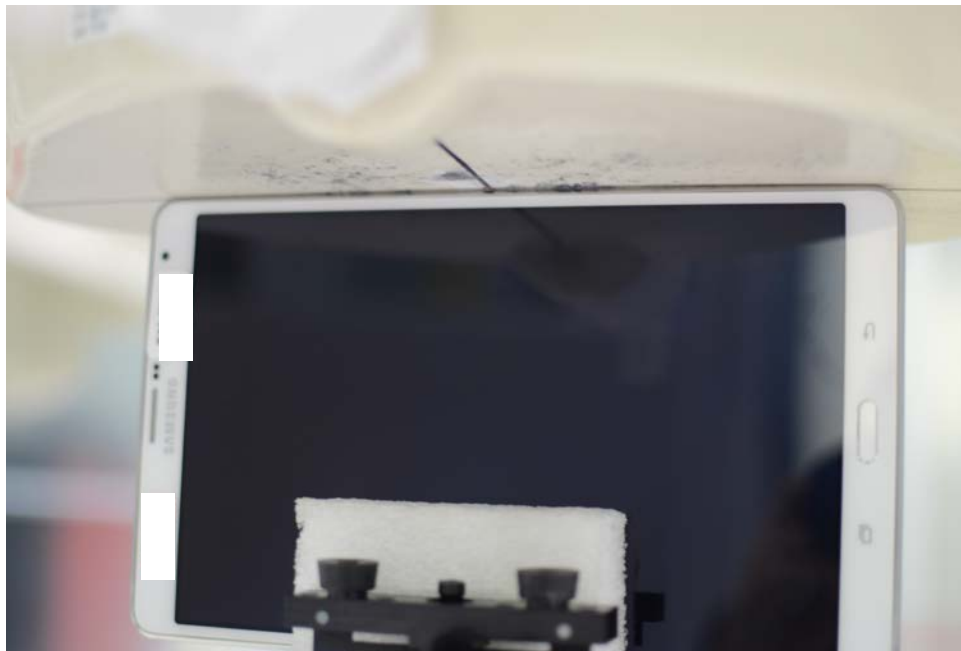
SAR Test Setup Photo 10 – Right Edge at 0 mm
