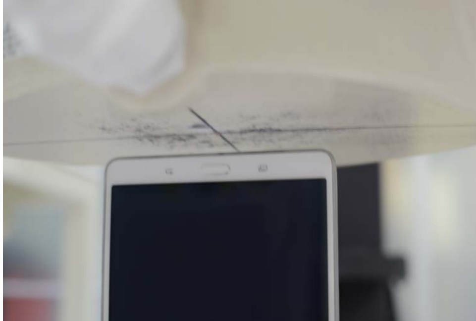
SAR Test Setup Photo 9 – Bottom Edge at 13 mm
