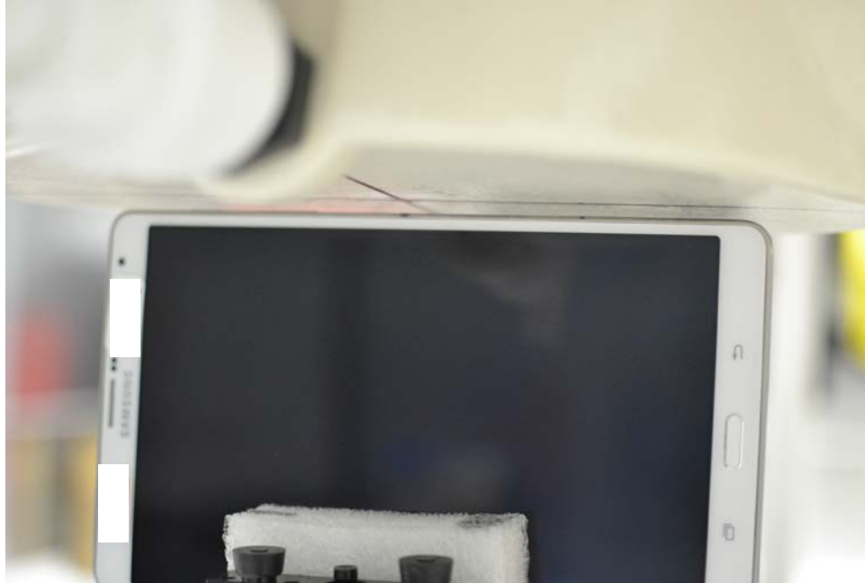
SAR Test Setup Photo 11 – Right Edge at 9 mm
