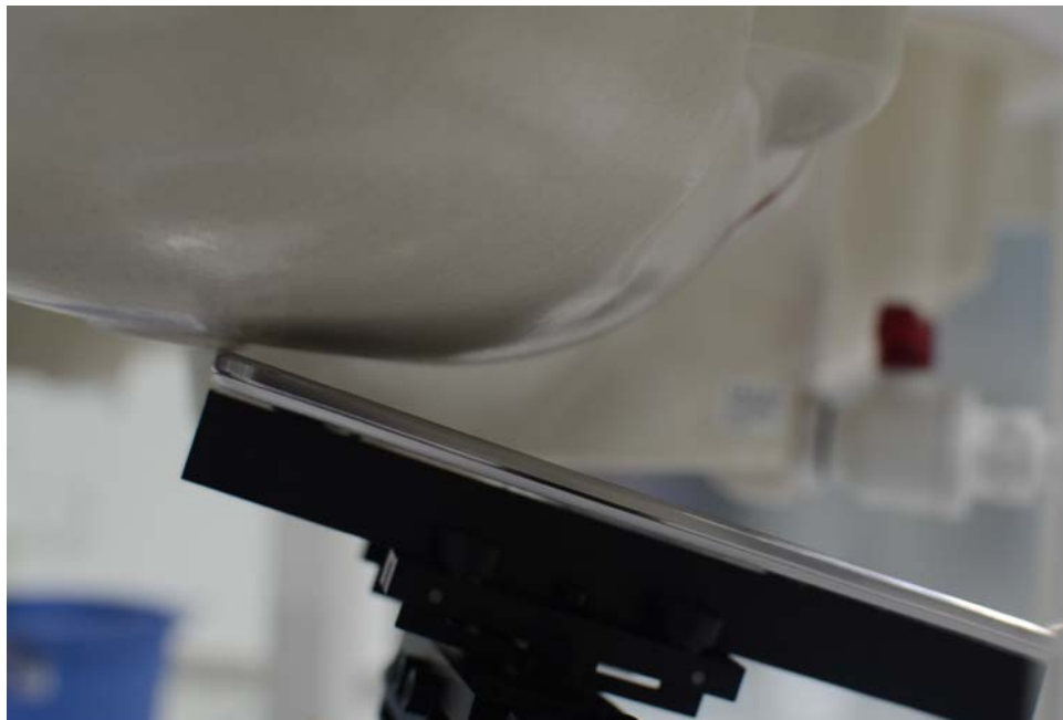
SAR Test Setup Photo 2 – Right Tilt
