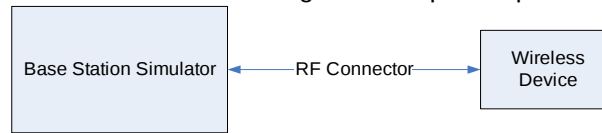
Figure 8-1 Power Measurement Setup
