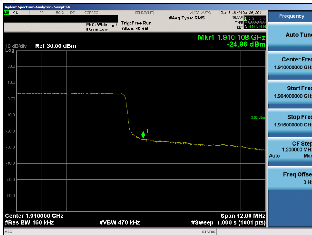
Plot 6-135. Upper Band Edge Plot (Band 2 – 15.0MHz QPSK – RB Size 75)
