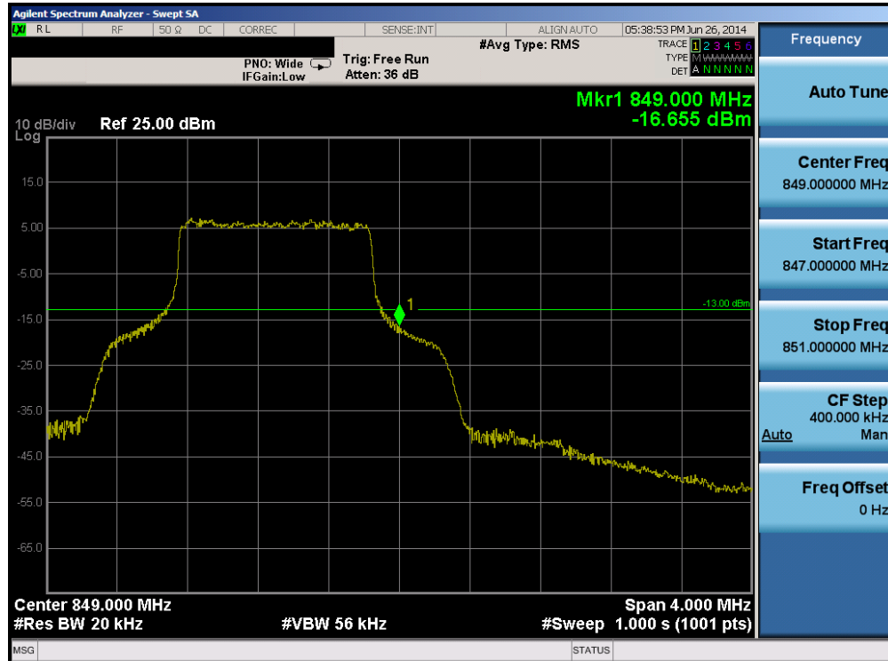
Plot 6-81. Upper Band Edge Plot (Band 5 – 1.4MHz QPSK – RB Size 6)
