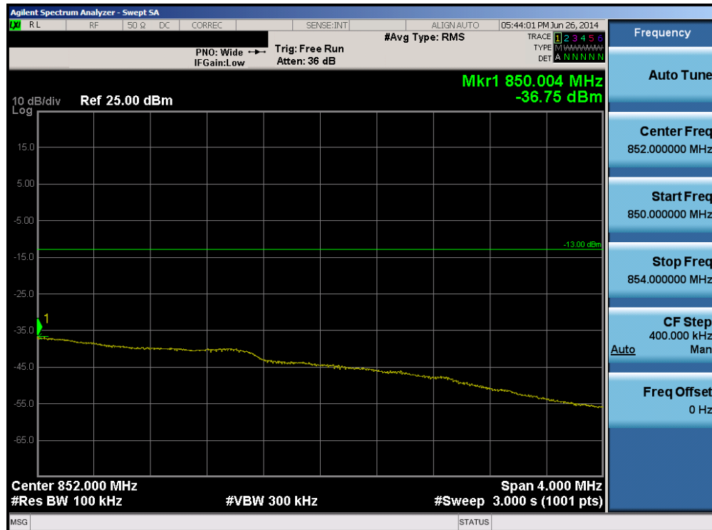
Plot 6-86. Upper Extended Band Edge Plot (Band 5 – Band 5 – 3.0MHz QPSK – RB Size 15)
