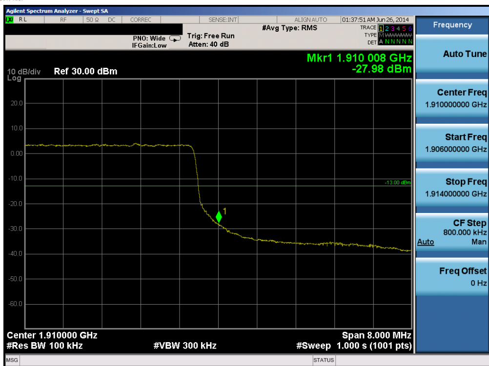
Plot 6-131. Upper Band Edge Plot (Band 2 – 10.0MHz QPSK – RB Size 50)
