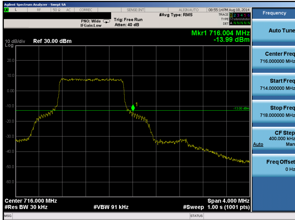
Plot 6-67. Upper Band Edge Plot (Band 12 – 1.4MHz QPSK – RB Size 6)
