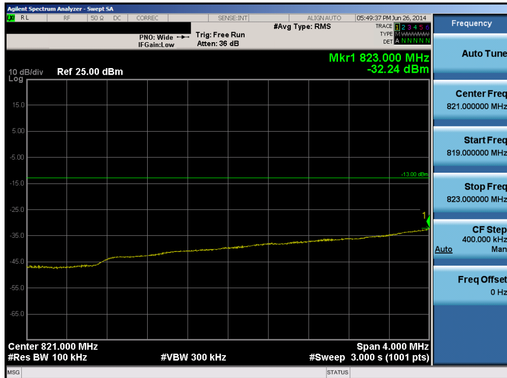
Plot 6-88. Lower Extended Band Edge Plot (Band 5 – 5.0MHz QPSK – RB Size 25)
