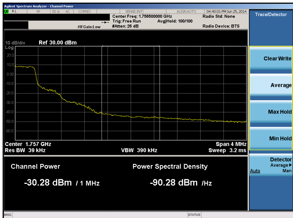
Plot 6-96. Upper Extended Band Edge Plot (Band 4 – 1.4MHz QPSK – RB Size 6)
