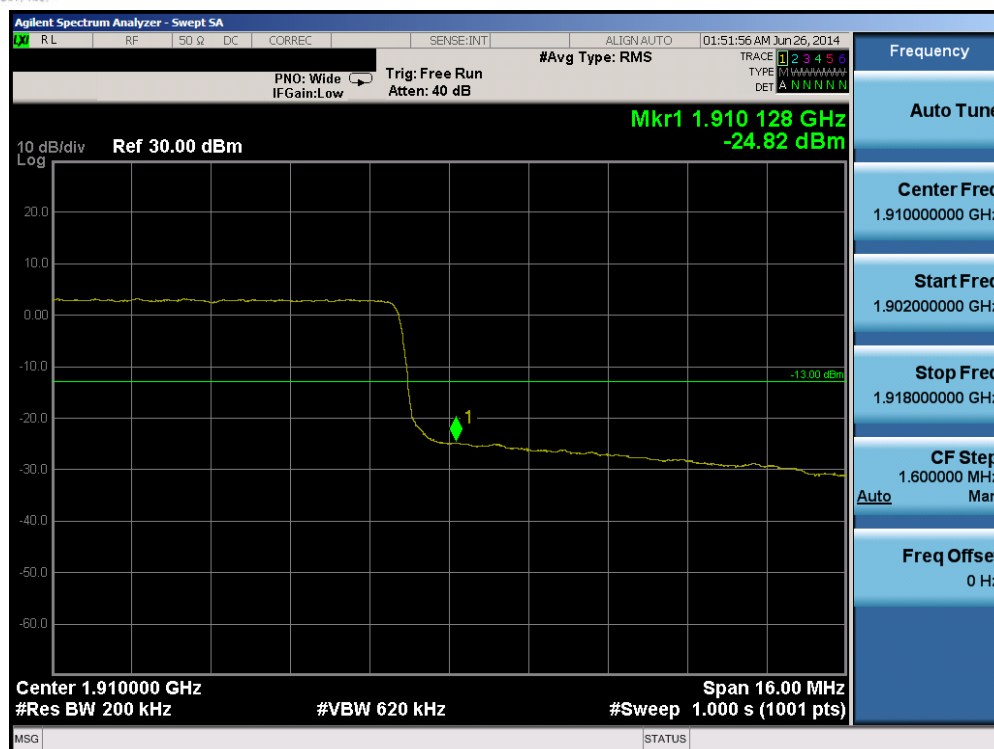
Plot 6-139. Upper Band Edge Plot (Band 2 – 20.0MHz QPSK – RB Size 100)
