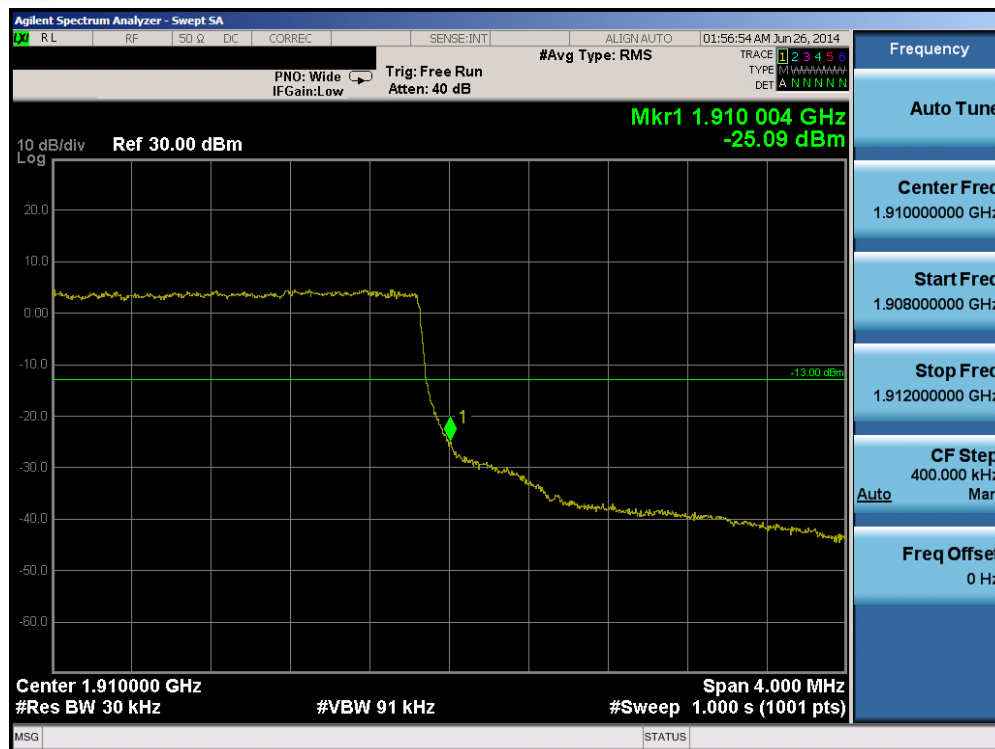
Plot 6-123. Upper Band Edge Plot (Band 2 – 3.0MHz QPSK – RB Size 15)
