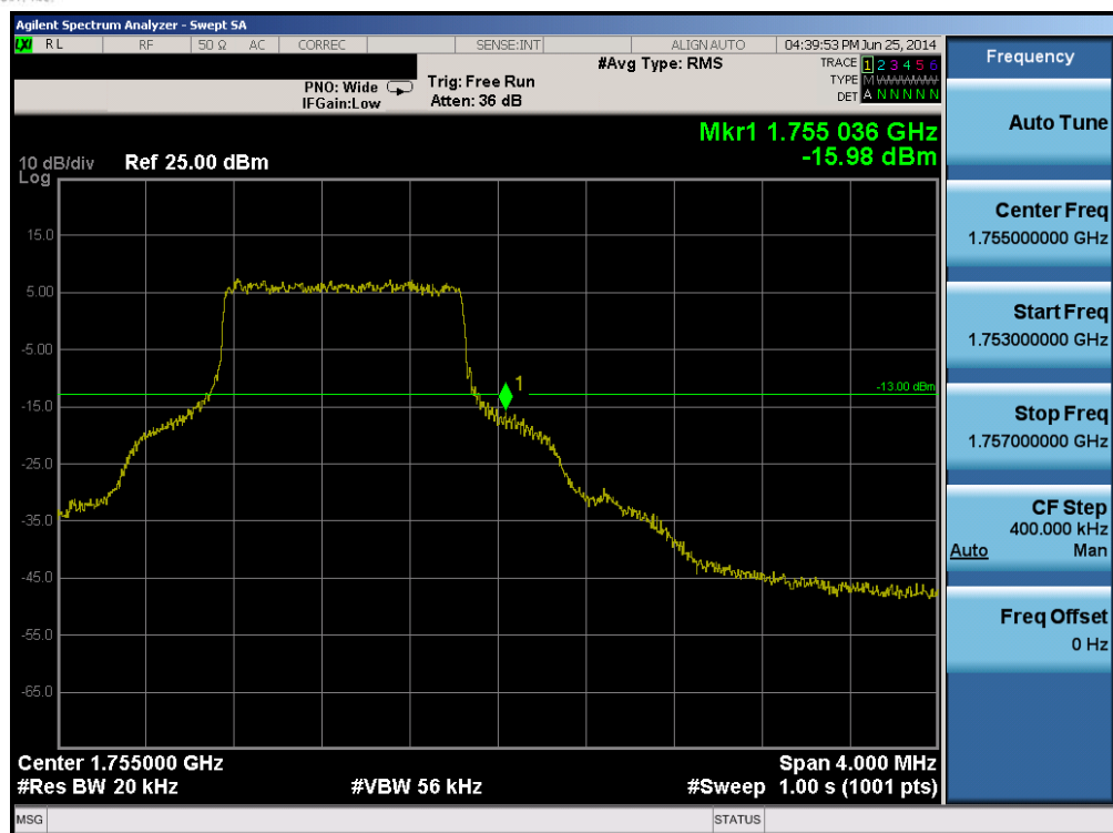
Plot 6-95. Upper Band Edge Plot (Band 4 – 1.4MHz QPSK – RB Size 6)
