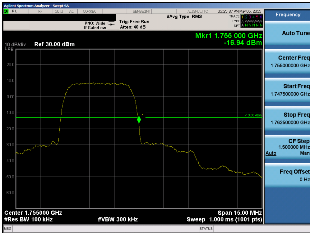
Plot 6-36. Band Edge Plot (AWS WCDMA Mode – Ch. 1862)
