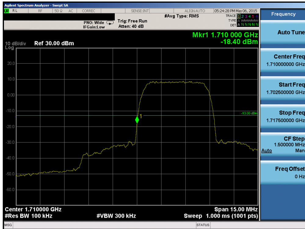
Plot 6-34. Band Edge Plot (AWS WCDMA Mode – Ch. 1312)
