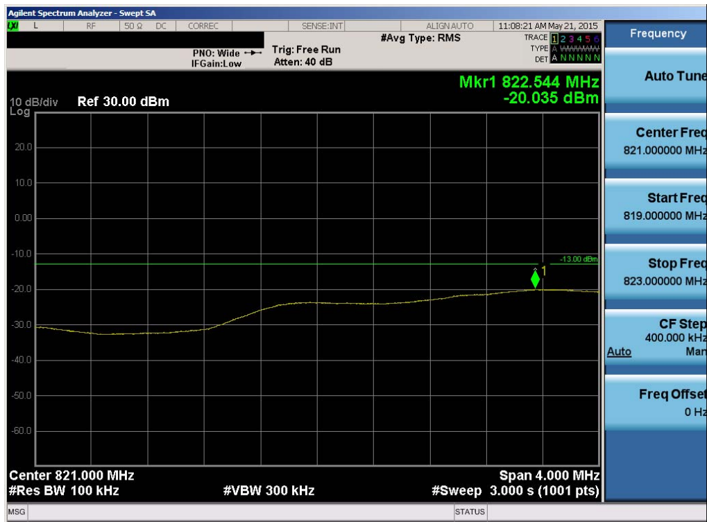
Plot 6-32. 4MHz Span Plot (Cellular WCDMA Mode – Ch. 4132)
