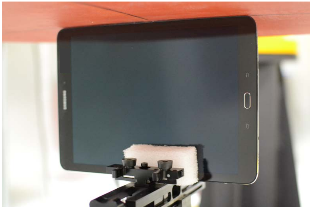
SAR Test Setup Photo 8: Right Edge at 0.0 cm
