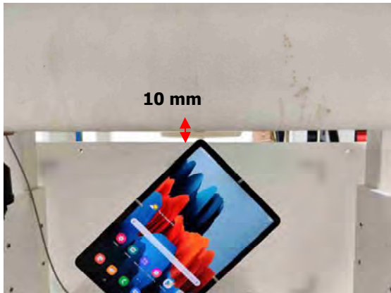
Fig.13 EUT Left corner side to flat phantom
