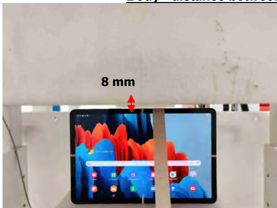
Fig.11 EUT Right side to flat phantom
