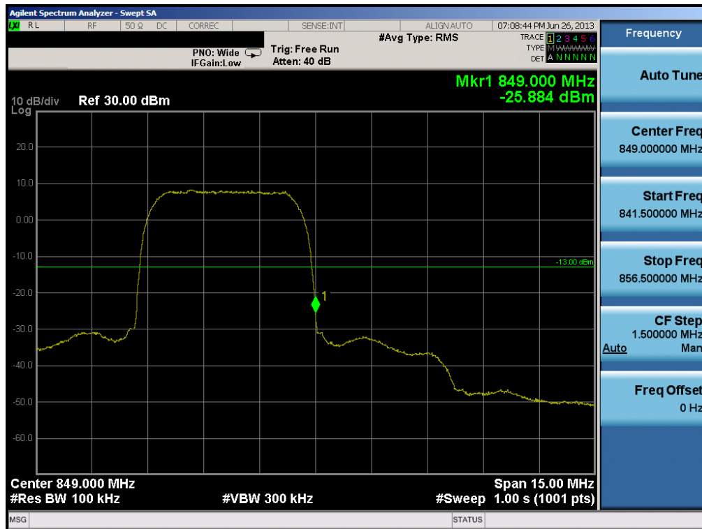
Plot 6-46. Band Edge Plot (Cellular WCDMA Mode – Ch. 4233)
