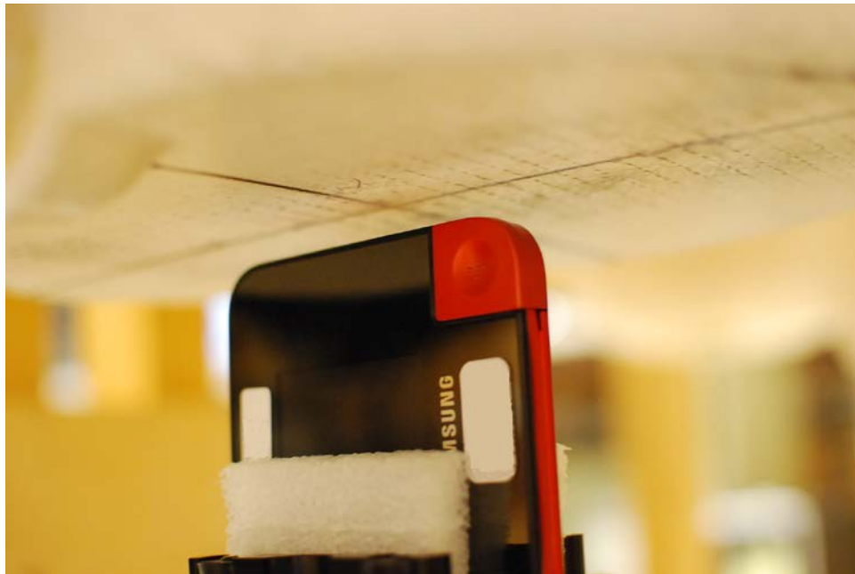
SAR Test Setup Photo 4 - Right Edge at 10 mm
