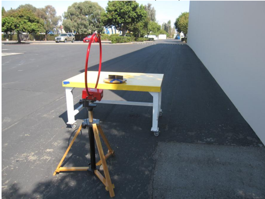
RADIATED EMISSIONS BELOW 30MHz (BACK)
