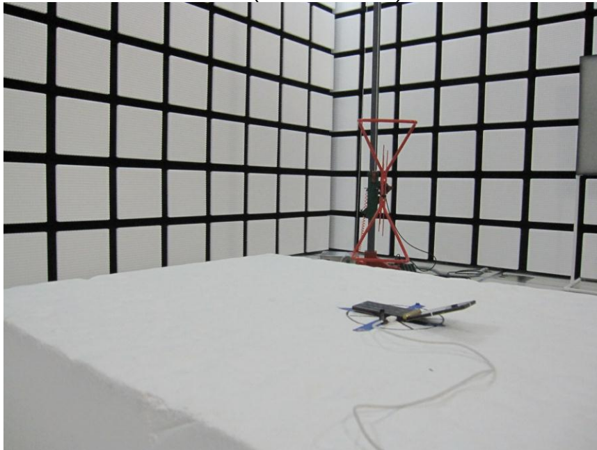
RADIATED BACK PHOTO (BELOW 1 GHz)
