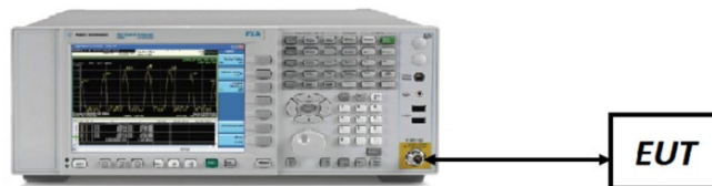
Figure 7-2. Test Instrument & Measurement Setup
