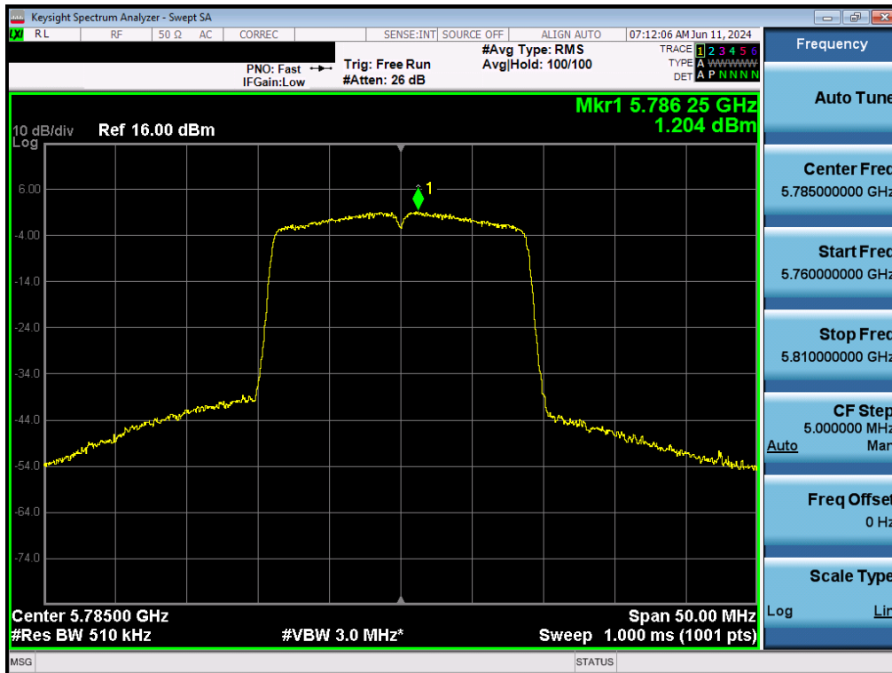
Plot 7-151. Power Spectral Density Plot MIMO ANT2 (20MHz BW 802.11n (UNII Band 3) – Ch. 157)
