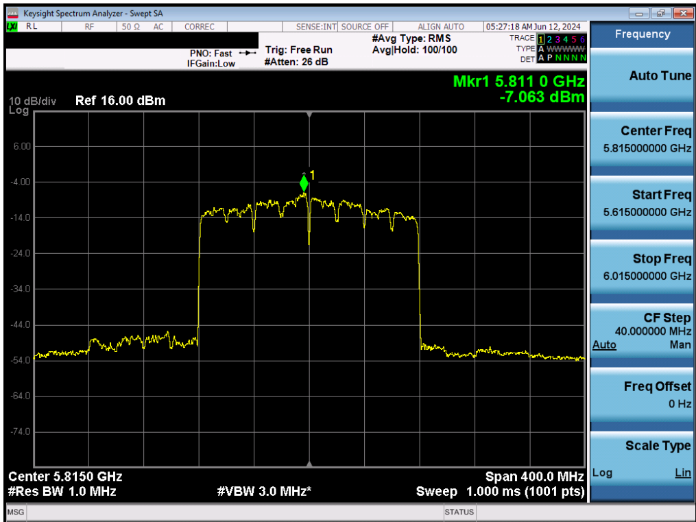
Plot 7-165. Power Spectral Density Plot MIMO ANT2 (160MHz BW 802.11ax (UNII Band 3/4) – Ch. 163)
