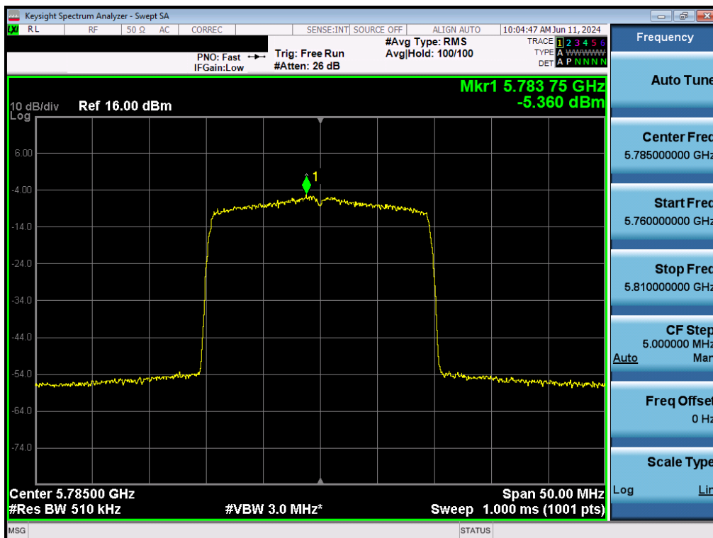
Plot 7-152. Power Spectral Density Plot MIMO ANT2 (20MHz BW 802.11ax (UNII Band 3) – Ch. 157)
