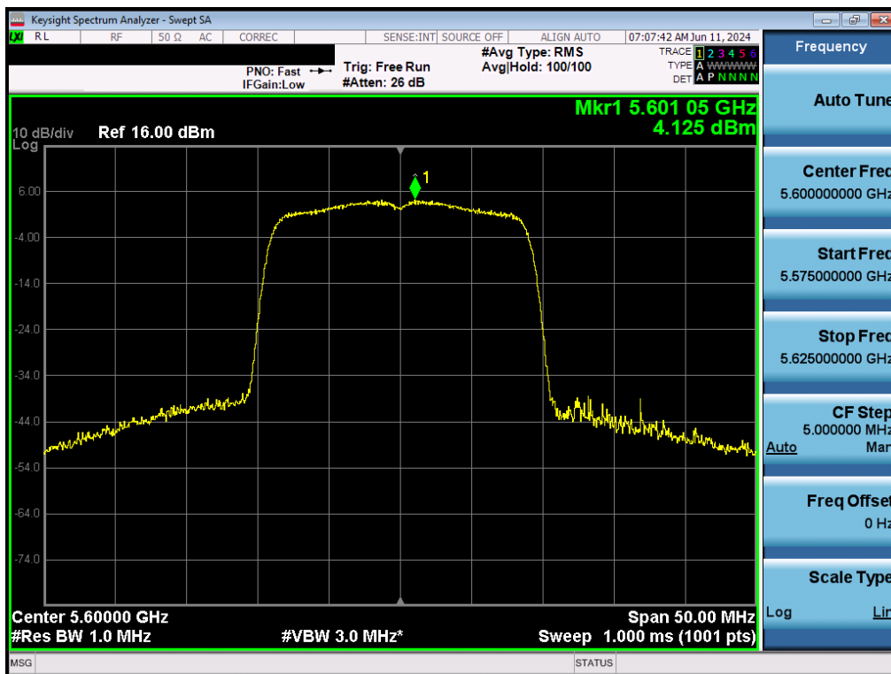
Plot 7-142. Power Spectral Density Plot MIMO ANT2 (20MHz BW 802.11n (UNII Band 2C) – Ch. 120)
