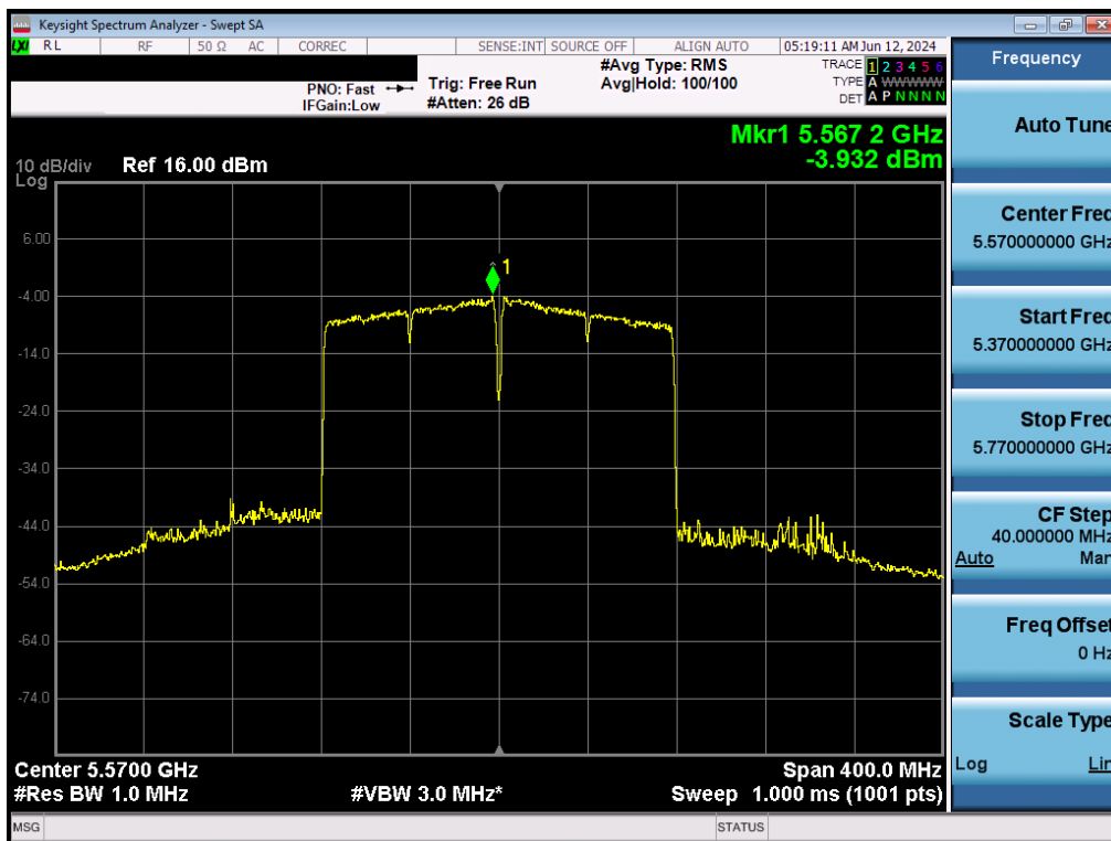
Plot 7-148. Power Spectral Density Plot MIMO ANT2 (160MHz BW 802.11ac (UNII Band 2C) – Ch. 114)
