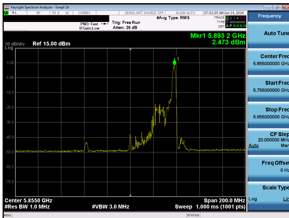
Plot 7-126. Power Spectral Density Plot MIMO ANT2 (80MHz BW 802.11ax – 26 Tones (UNII Band 3/4) – Ch. 171)
