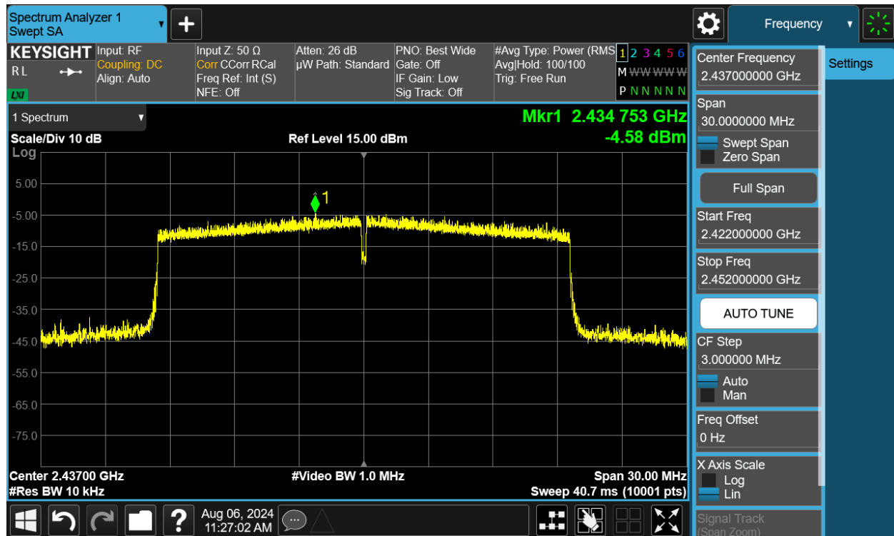
Plot 7-83. Power Spectral Density Plot MIMO ANT1 (802.11be (2.4GHz) – Ch. 6)
