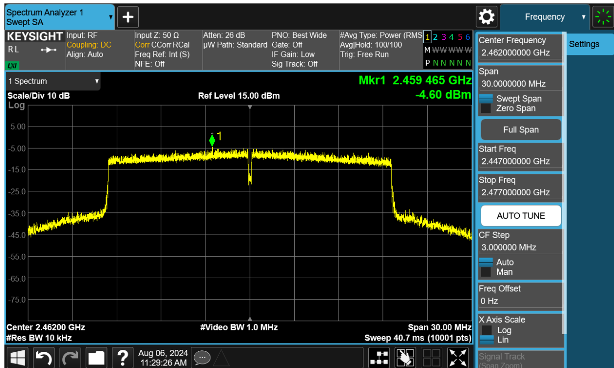
Plot 7-84. Power Spectral Density Plot MIMO ANT1 (802.11be (2.4GHz) – Ch. 11)
