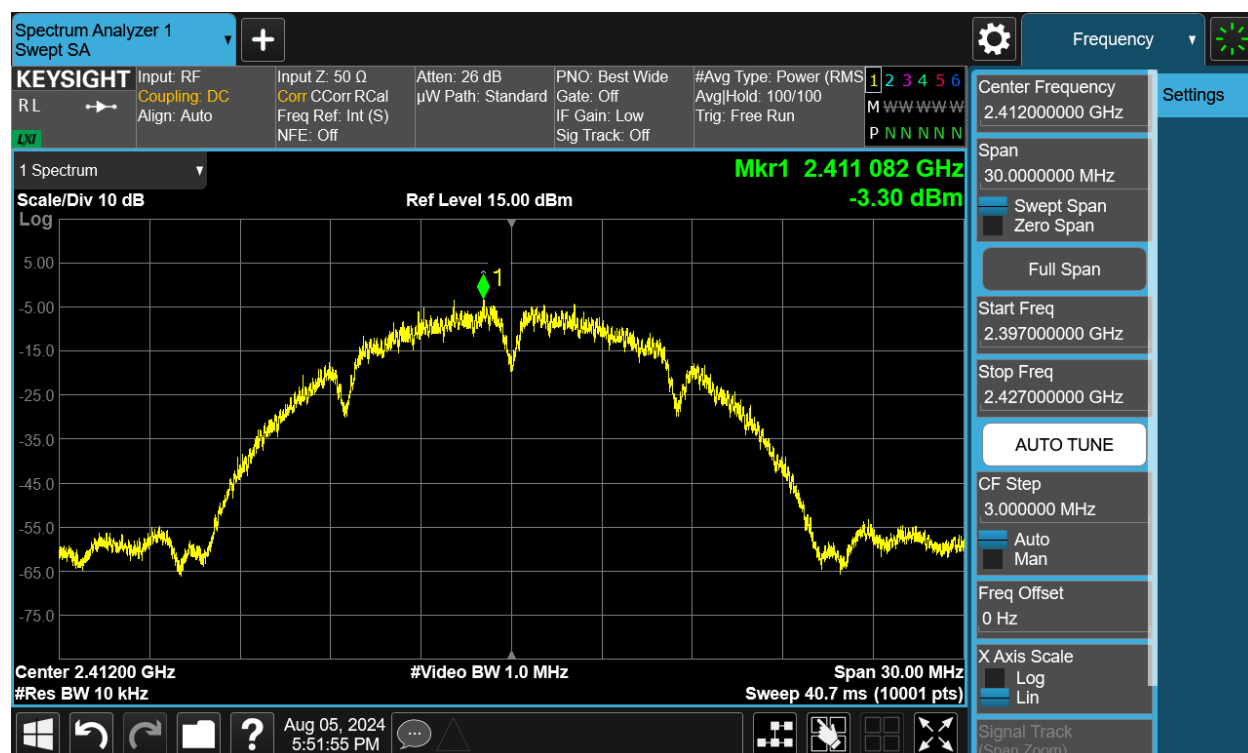
Plot 7-73. Power Spectral Density Plot MIMO ANT1 (802.11b – Ch. 1)
