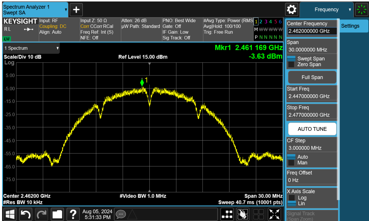
Plot 7-51. Power Spectral Density Plot SISO ANT1 (802.11b – Ch. 11)
