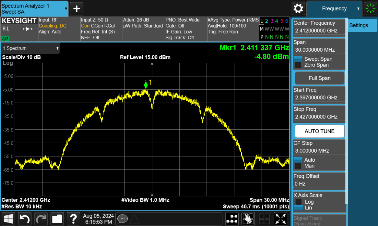
Plot 7-85. Power Spectral Density Plot MIMO ANT2 (802.11b – Ch. 1)
