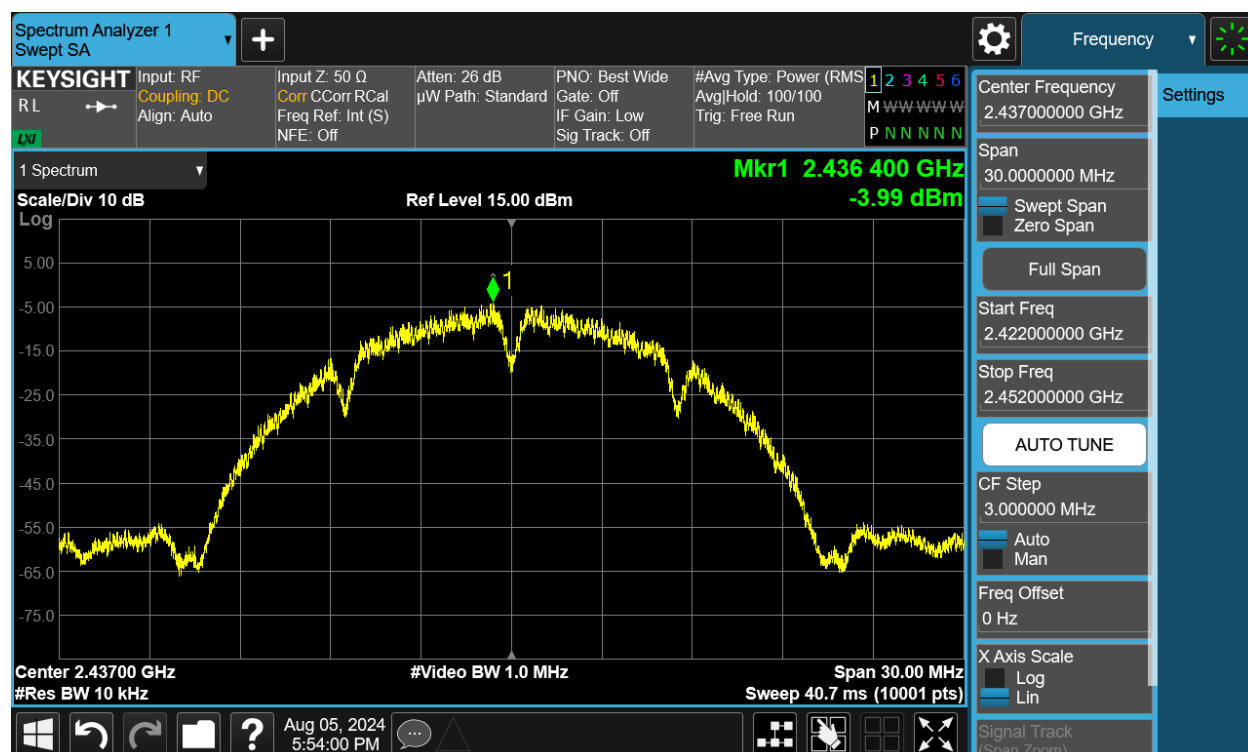
Plot 7-74. Power Spectral Density Plot MIMO ANT1 (802.11b – Ch. 6)
