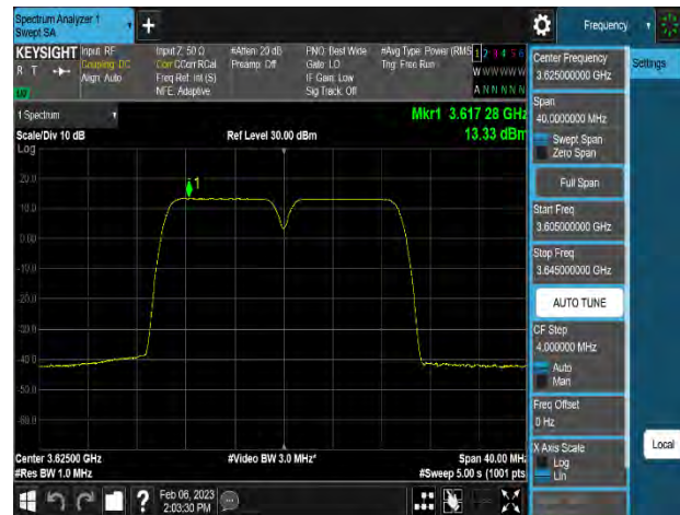
Plot 8-44. Power Spectral Density Plot (n48_2C_10M+10M_QPSK - Mid Channel_8T, Port 2)
