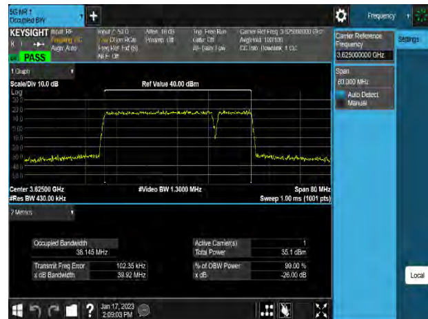
Plot 8-16. Occupied Bandwidth Plot (n48_2C_30M+10M_16QAM - Mid Channel, Port 1)
