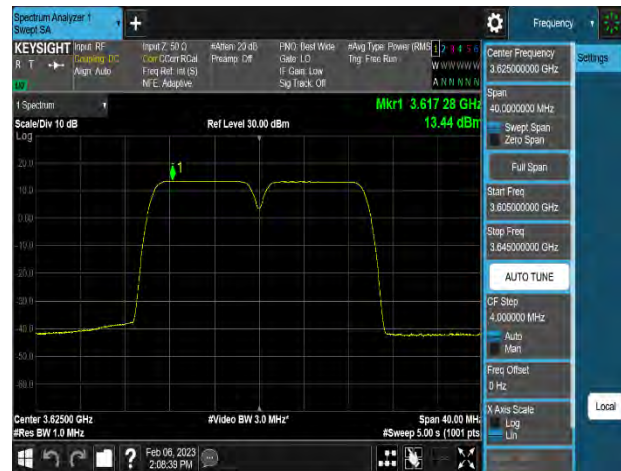
Plot 8-50. Power Spectral Density Plot (n48_2C_10M+10M_QPSK - Mid Channel_8T, Port 8)
