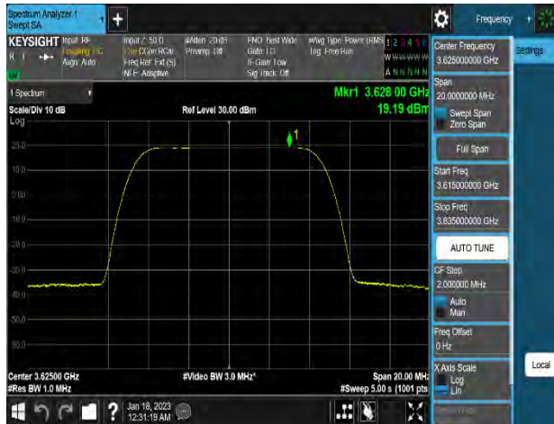
Plot 8-29. Power Spectral Density Plot (n48_1C_10M_256QAM - Mid Channel_4T, Port 7)
