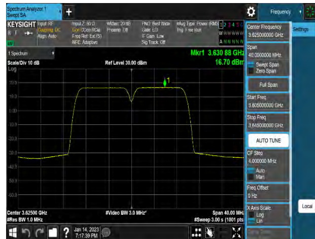
Plot 8-26. Power Spectral Density Plot (n48_2C_10M+10M_16QAM - Mid Channel_2T, Port 6)
