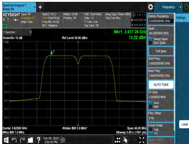
Plot 8-43. Power Spectral Density Plot (n48_2C_10M+10M_QPSK - Mid Channel_8T, Port 1)
