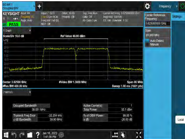
Plot 8-13. Occupied Bandwidth Plot (n48_2C_20M+20M_QPSK - Mid Channel, Port 1)
