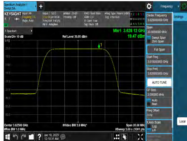
Plot 8-24. Power Spectral Density Plot (n48_1C_10M_16QAM - Mid Channel_2T, Port 6)
