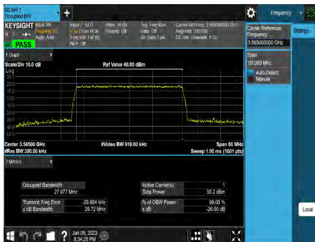
Plot 8-5. Occupied Bandwidth Plot (n48_1C_30M_QPSK - Low Channel, Port 4)
