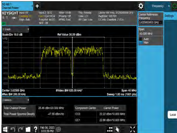
Plot 8-224. Equivalent Isotropic Radiated Power Plot (n48_2C_10M+10M_16QAM - Mid Channel_8T, Port 1)
