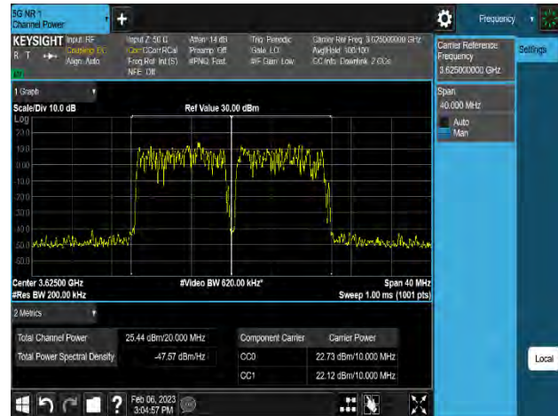
Plot 8-225. Equivalent Isotropic Radiated Power Plot (n48_2C_10M+10M_16QAM - Mid Channel_8T, Port 2)
