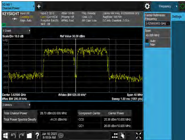
Plot 8-213. Equivalent Isotropic Radiated Power Plot (n48_2C_10M+10M_16QAM – Mid Channel_2T, Port 5)
