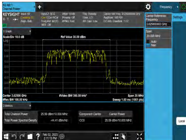
Plot 8-220. Equivalent Isotropic Radiated Power Plot (n48_1C_10M_QPSK - Mid Channel_8T, Port 5)
