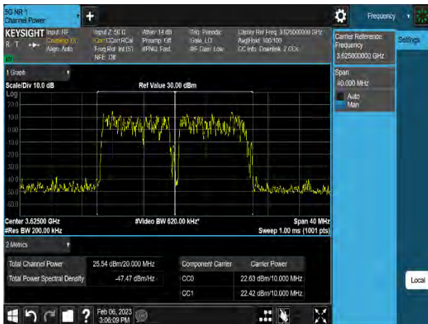
Plot 8-226. Equivalent Isotropic Radiated Power Plot (n48_2C_10M+10M_16QAM - Mid Channel_8T, Port 3)
