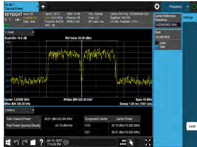
Plot 8-214. Equivalent Isotropic Radiated Power Plot (n48_2C_10M+10M_16QAM – Mid Channel_2T, Port 6)
