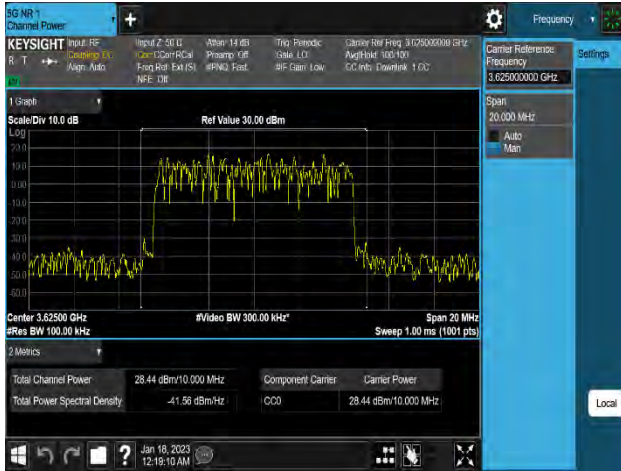
Plot 8-211. Equivalent Isotropic Radiated Power Plot (n48_1C_10M_256QAM – Mid Channel_2T, Port 5)
