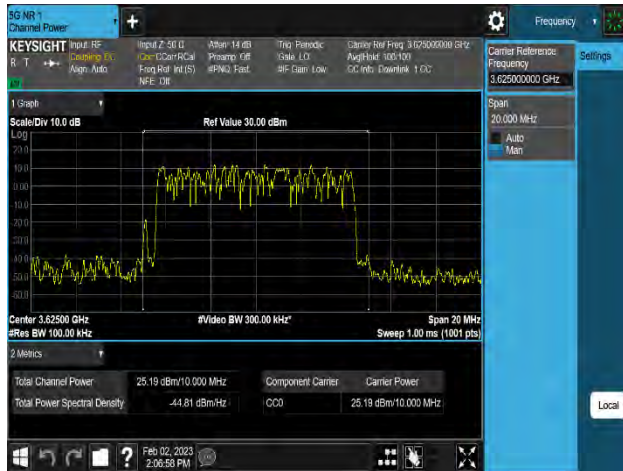
Plot 8-216. Equivalent Isotropic Radiated Power Plot (n48_1C_10M_QPSK - Mid Channel_8T, Port 1)
