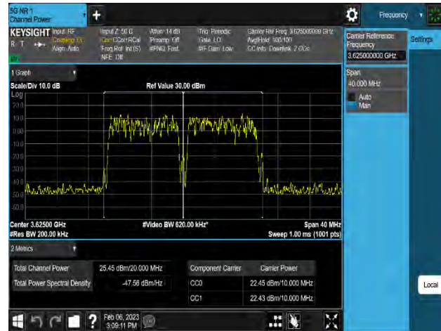
Plot 8-229. Equivalent Isotropic Radiated Power Plot (n48_2C_10M+10M_16QAM - Mid Channel_8T, Port 6)
