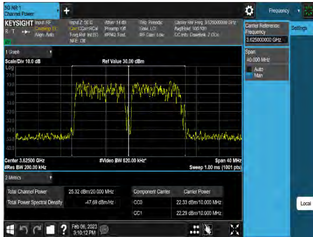
Plot 8-230. Equivalent Isotropic Radiated Power Plot (n48_2C_10M+10M_16QAM - Mid Channel_8T, Port 7)
