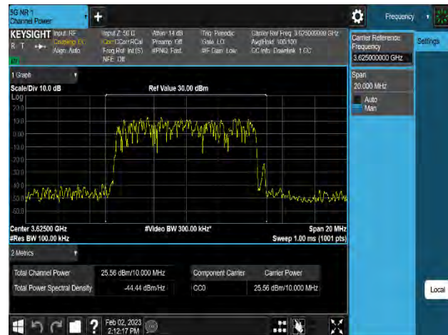
Plot 8-221. Equivalent Isotropic Radiated Power Plot (n48_1C_10M_QPSK - Mid Channel_8T, Port 6)
