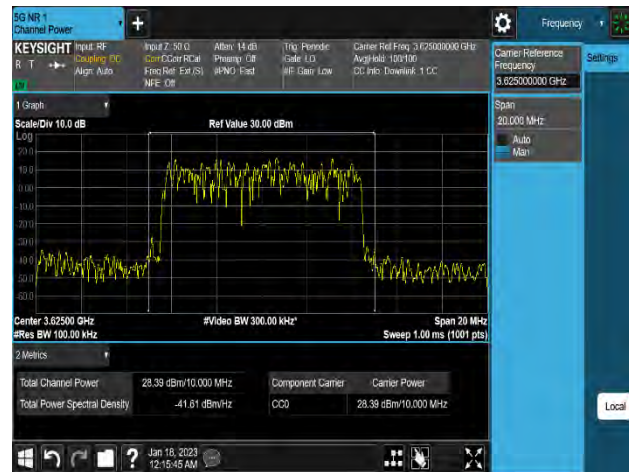
Plot 8-211. Equivalent Isotropic Radiated Power Plot (n48_1C_10M_256QAM – Mid Channel_4T, Port 6)
