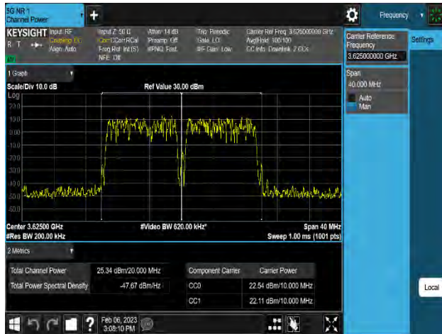
Plot 8-228. Equivalent Isotropic Radiated Power Plot (n48_2C_10M+10M_16QAM - Mid Channel_8T, Port 5)
