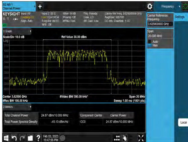
Plot 8-218. Equivalent Isotropic Radiated Power Plot (n48_1C_10M_QPSK - Mid Channel_8T, Port 3)
