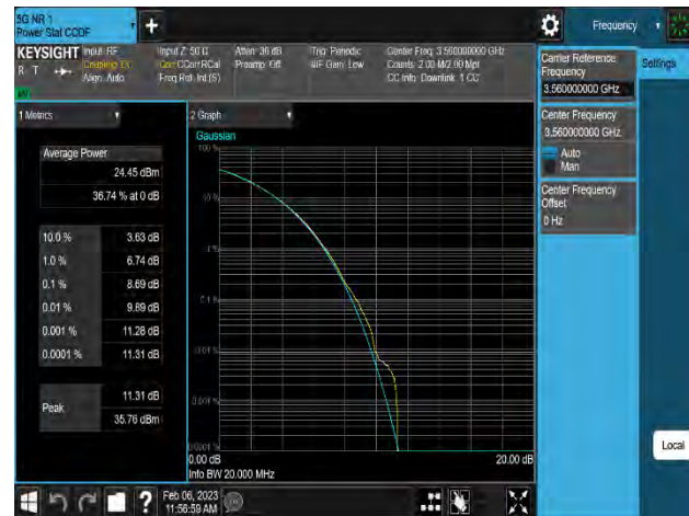
Plot 8-241. Peak To Average Power Ratio Plot (n48_2C_10M+10M_QPSK - Low Channel, Port 1_8TX)
