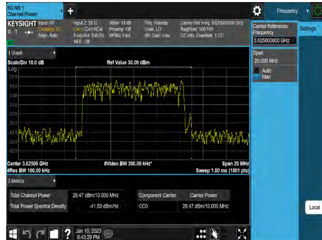
Plot 8-211. Equivalent Isotropic Radiated Power Plot (n48_1C_10M_256QAM – Mid Channel_4T, Port 8)
