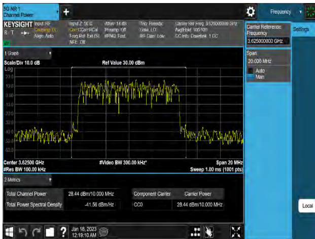
Plot 8-211. Equivalent Isotropic Radiated Power Plot (n48_1C_10M_256QAM – Mid Channel_4T, Port 5)
