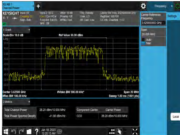
Plot 8-211. Equivalent Isotropic Radiated Power Plot (n48_1C_10M_256QAM – Mid Channel_4T, Port 7)
