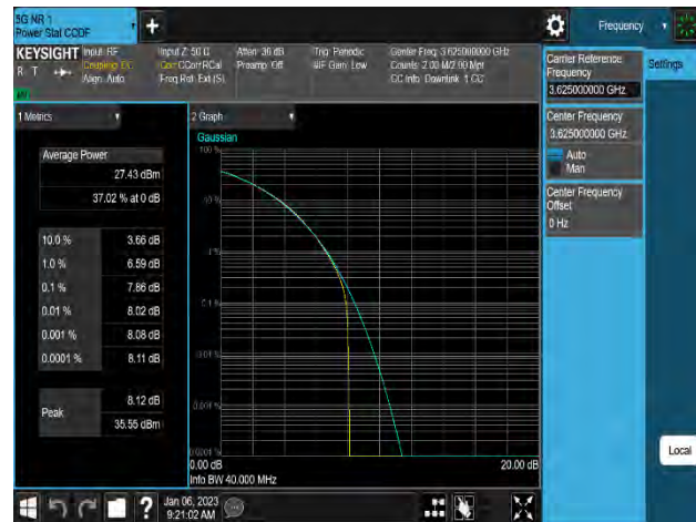
Plot 8-235. Peak To Average Power Ratio Plot (n48_1C_40M_16QAM - Mid Channel, Port 1_2TX)
