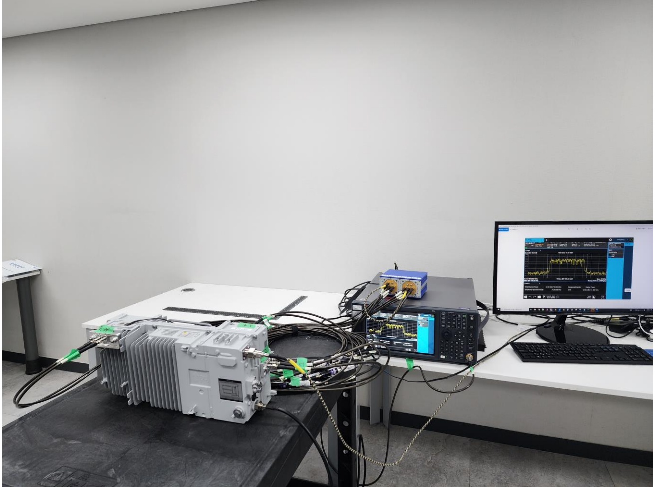
Conducted Test Instrument & Measurement Setup
