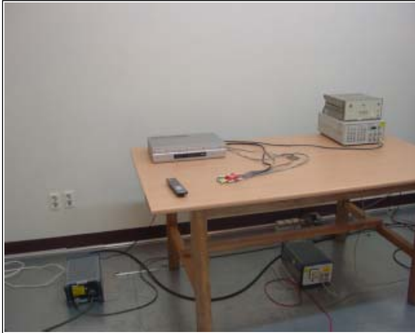
AC Powerline Conducted Emission [Front]
