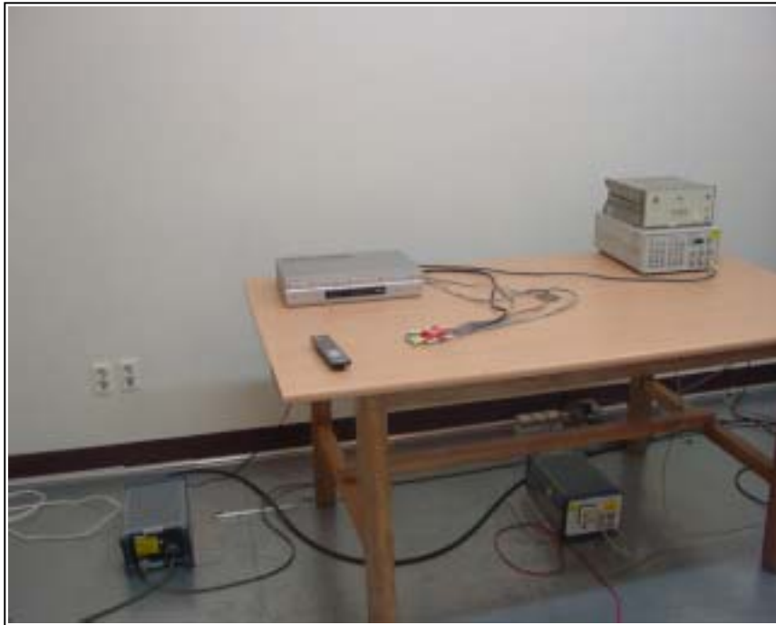
AC Powerline Conducted Emission [Front]
