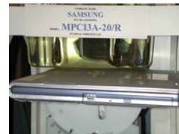
Figure 14.1 DSSS Body SAR Test Setup
