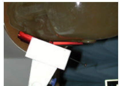
Figure 14. Head SAR Test Setup
