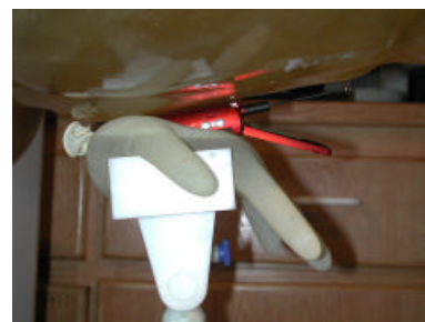
Figure 16. Hand SAR Test Setup
