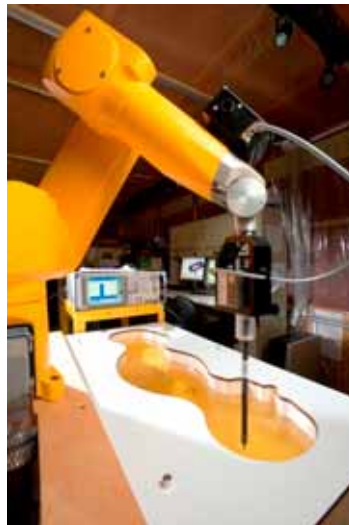
Figure 3-2 DASY4 SAR Measurement System
