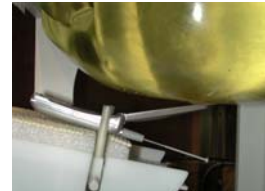
Figure 14.11 Left Head SAR Test Setup -- Ear / Tilt Position --
