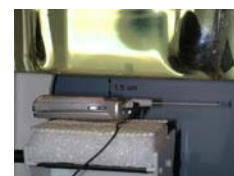
Figure 14.14 Body SAR Test Setup -- w/o Holster --
