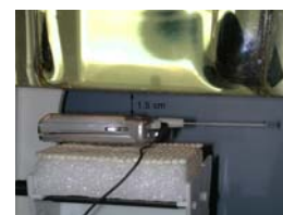
Figure 14.13 Body SAR Test Setup -- w/o Holster --
