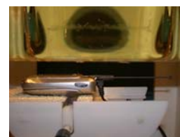
Figure 14.15 Body SAR Test Setup -- w/o Holster --
