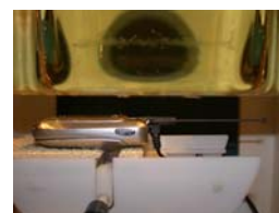
Figure 14.14 Body SAR Test Setup -- w/o Holster --
