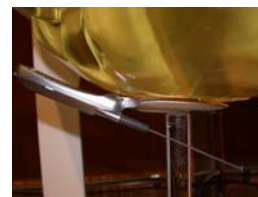
Figure 14.7 Right Head SAR Test Setup -- Cheek / Touch Position --
