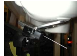
Figure 14.9 Left Head SAR Test Setup -- Ear / Tilt Position --
