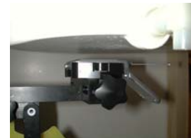
Figure 14.12 Body SAR Test Setup -- w/o Holster --
