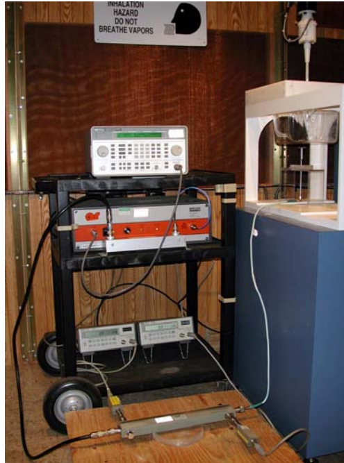
Figure 7.1 – Test system for the system performance check
