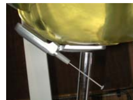
Figure 14.4 Left Head SAR Test Setup -- Cheek / Touch Position --
