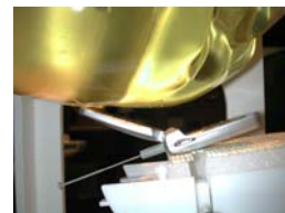
Figure 14.6 Right Head SAR Test Setup -- Ear / 15° Tilt Position --
