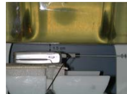
Figure 14.11 Body SAR Test Setup -- w/o Holster --
