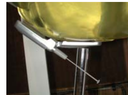
Figure 14.8 Left Head SAR Test Setup -- Cheek / Touch Position --
