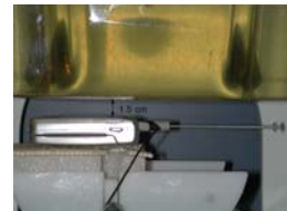
Figure 14.12 Body SAR Test Setup -- w/o Holster --
