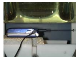
Figure 14.12 Body SAR Test Setup -- w/o Holster --
