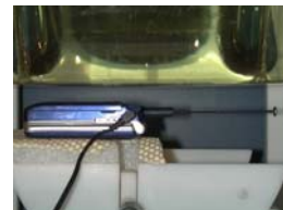
Figure 14.11 Body SAR Test Setup -- w/o Holster --
