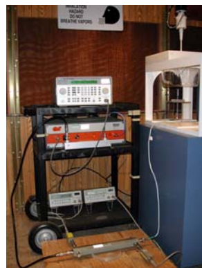
Figure 12.1 Dipole Validation Test Setup
