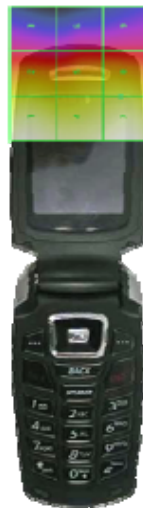
Figure 28 Sample H-field Scan Overlay
