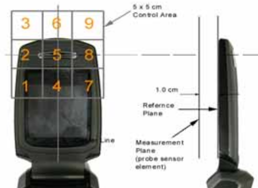
Figure 13 E/H-Field Emissions Test Setup Diagram
