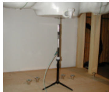
Figure 12.1 Dipole Validation Test Setup
