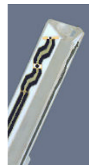
Figure 3.2 Probe Thick-Film Technique
