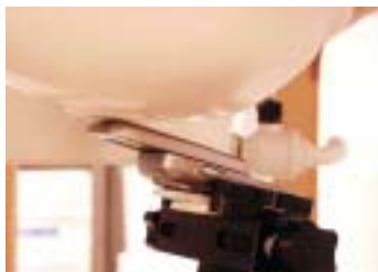
Figure 8.11 Right Head SAR Test Setup -- Ear/Tilt 15° Position--
