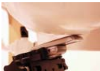
Figure 8.13 Left Head SAR Test Setup -- Ear/Tilt 15° Position--
