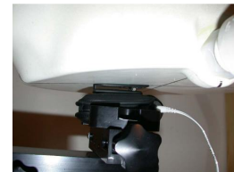
Figure 14.14 Body SAR Test Setup -- w/ Holster --
