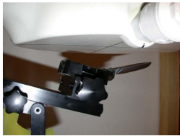
Figure 14.16 Face SAR Test Setup -- Flip Open --
