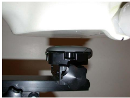
Figure 14.17 Face SAR Test Setup -- Flip Closed --
