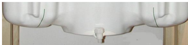
Figure 7.2 SAM Twin Phantom shell
