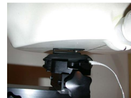
Figure 14.13 Body SAR Test Setup -- w/ Holster --
