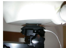
Figure 14.15 Body SAR Test Setup -- w/ Belt-clip --
