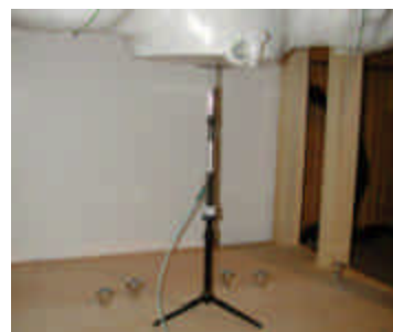
Figure 12.1 Dipole Validation Test Setup
