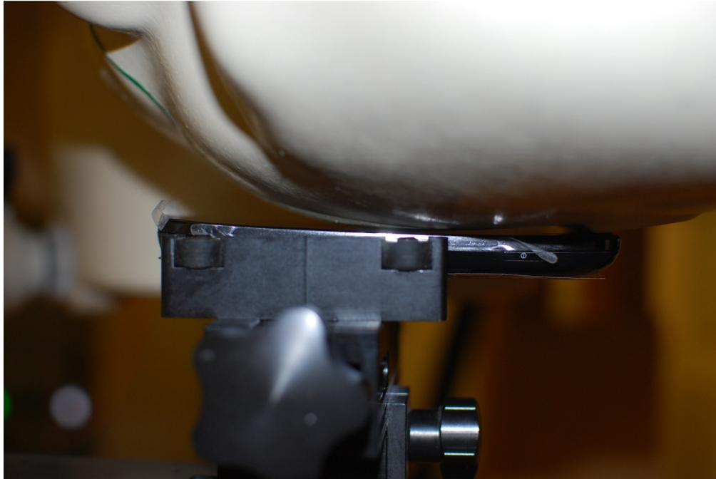
Figure 24-3 SAR Test Setup Photo – Left Touch
