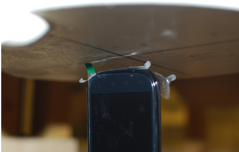
Figure 24-8 SAR Test Setup Photo – Bottom Edge at 1.0cm
