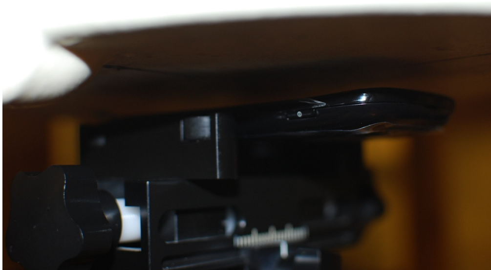
Figure 24-6 SAR Test Setup Photo – Front at 1.0cm
