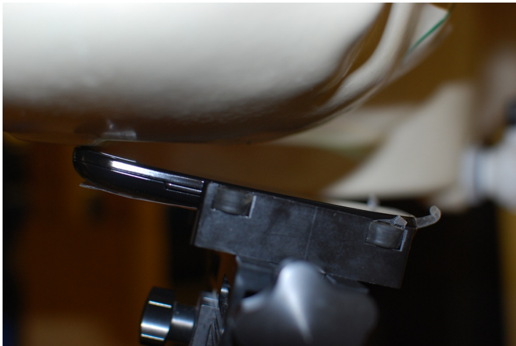
Figure 24-2 SAR Test Setup Photo – Right Tilt
