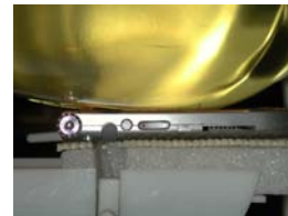
Figure 14.7 Right Head SAR Test Setup -- Cheek / Touch Position --
