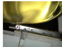
Figure 14.8 Right Head SAR Test Setup -- Ear / 15° Tilt Position --
