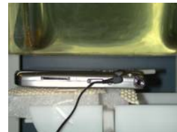
Figure 14.14 Body SAR Test Setup -- w/o Holster --
