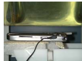
Figure 14.13 Body SAR Test Setup -- w/o Holster --
