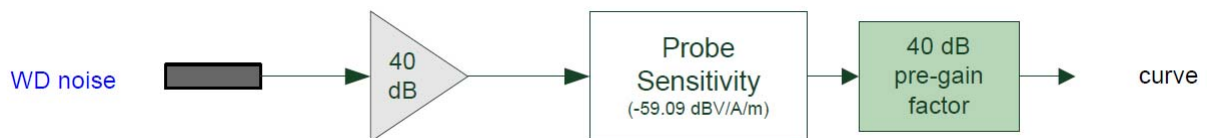
Figure 6-2 Audio Band Magnetic Curve Measurement Block Diagram
