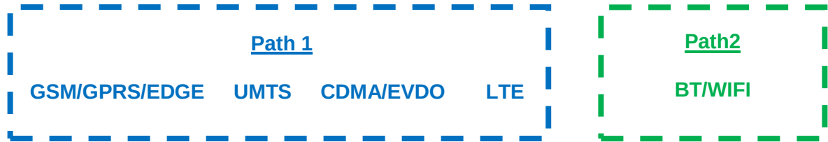
Figure 1-3 Simultaneous Transmission Paths
