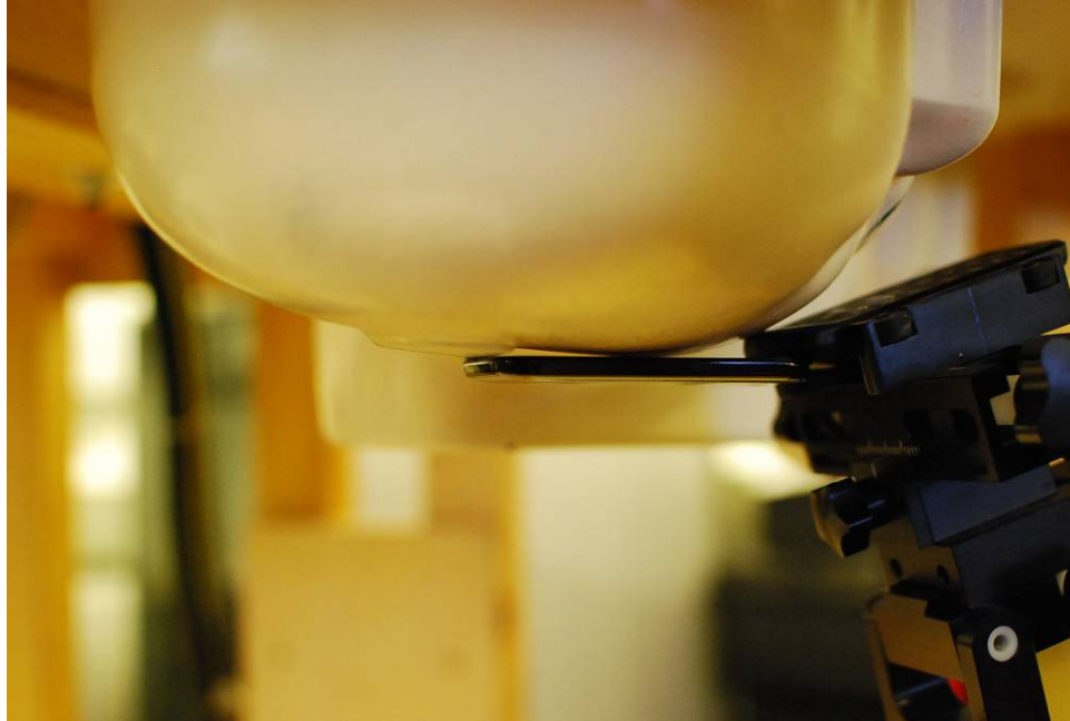
SAR Test Setup Photo 1 – Right Touch
