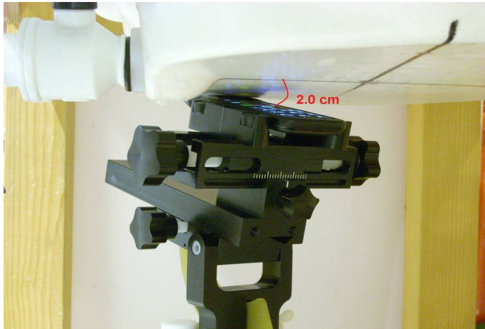
SAR Test Setup Photo 5 – Mouth-Jaw at 2.0 cm
