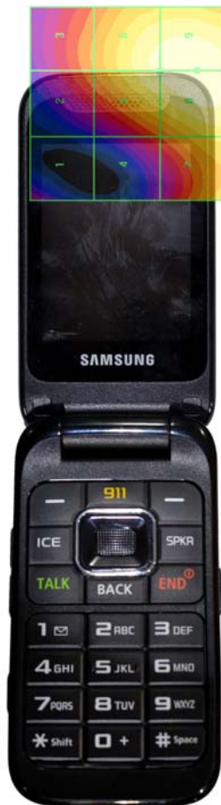
Figure 17-4 E-Field WD Scan overlay
