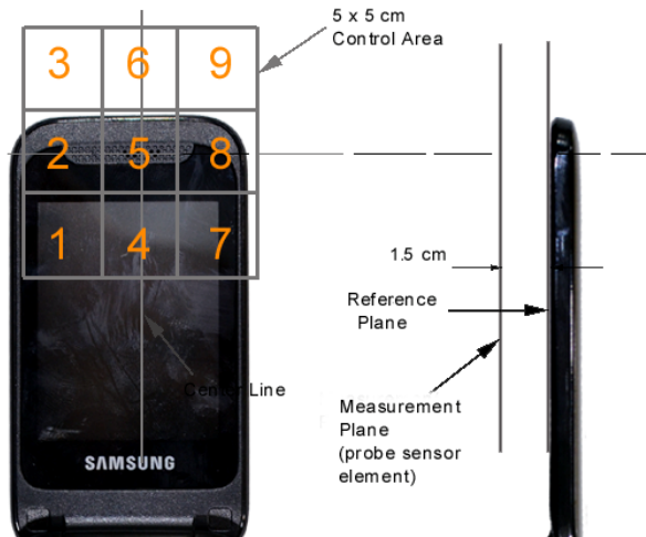
Figure 17-3 5x5 Scan grid above WD
