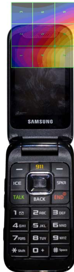
Figure 17-5 H-Field WD Scan overlay
