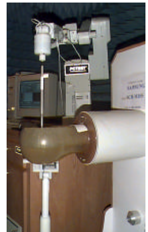
Figure 1. SAR Test Set-up
