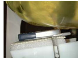
Figure 14.11 Left Head SAR Test Setup -- Ear / Tilt Position --
