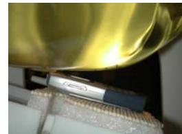
Figure 14.9 Right Head SAR Test Setup -- Ear / Tilt Position --
