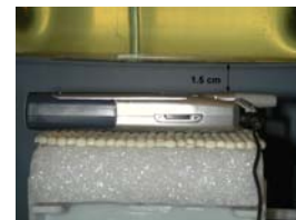
Figure 14.12 Body SAR Test Setup -- w/o Holster --
