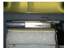
Figure 14.13 Body SAR Test Setup -- w/o Holster --
